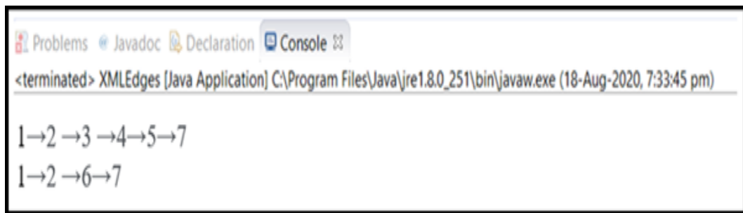
FIGURE 4.14: Test-Paths for the CFG E2 of the Tachometer Application
